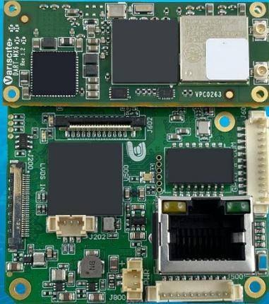
Red Mamba Neo IP video encoding module has been specifically designed for compact embedded vision systems.
